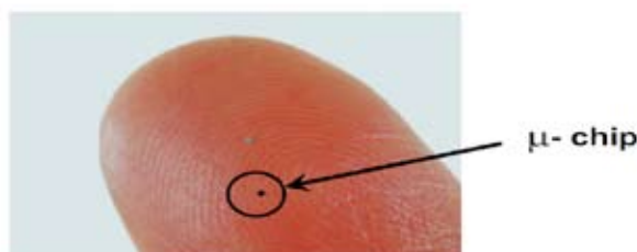
Figure 22. Hitachi's \mu -chip, one of the world's smallest RFID tags, measuring 0.4 x 0.4 mm
